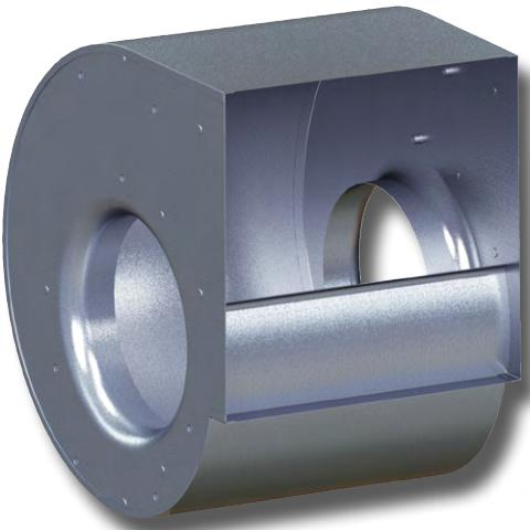
Twin City Fan & Blower air kits are provided with the forward curve design in the double-width, double-inlet arrangement. This design allows for a low operating speed and economically sized shafting. These air kits provide reliable and quiet operation in ovens and plenums where it is not desirable to have the fan bearings in the airstream. The air kit design is commonly used to economically provide large volumes of air (up to 100,000 CFM) at static pressures up to 6" w.g. in a compact design.
