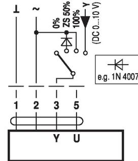
Control remotely 0...100% with positioner SG..
