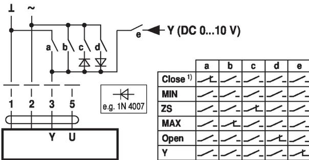
Override control and limiting with AC 24 V with rotary switch
