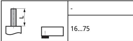
Clamping range damper shaft
