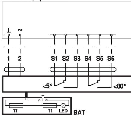
**Plug connection to communication and power supply units:**
