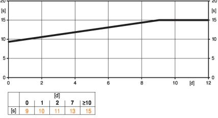
[d] = Electricity interruption in days [s] = Pre-charging time in seconds PF[s] = Bridging time
