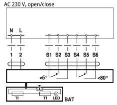
Plug connection to communication and power supply units:
