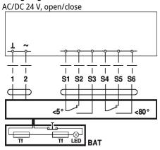
Plug connection to communication and power supply units:
